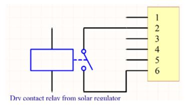
The SATS is triggered by an external signal such as an output from a solar charge controller. This trigger is to close Terminal 6 and 2 together.
